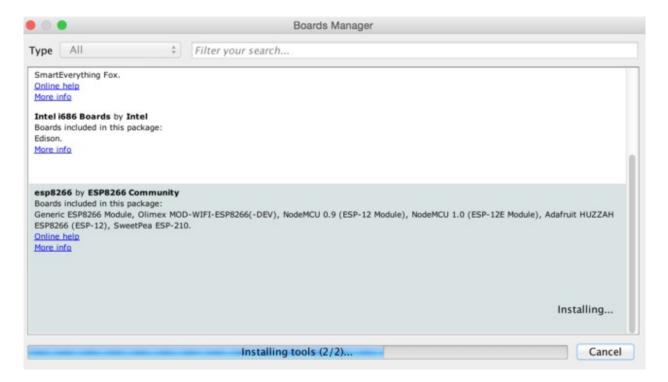
After the install process, you should see that esp8266 package is marked INSTALLED. Close the Boards Manager window once the install process has completed.
